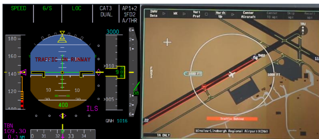
Figure 5: SURF-A/IA HMI in A320 / business jet cockpits
